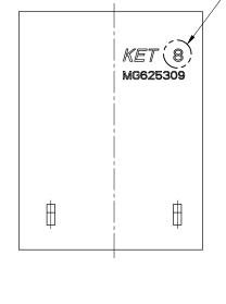
NO. PART NO. MATERIAL PBT (VO) MG625309 PET/PC (G.W.I.T) MG625309T
